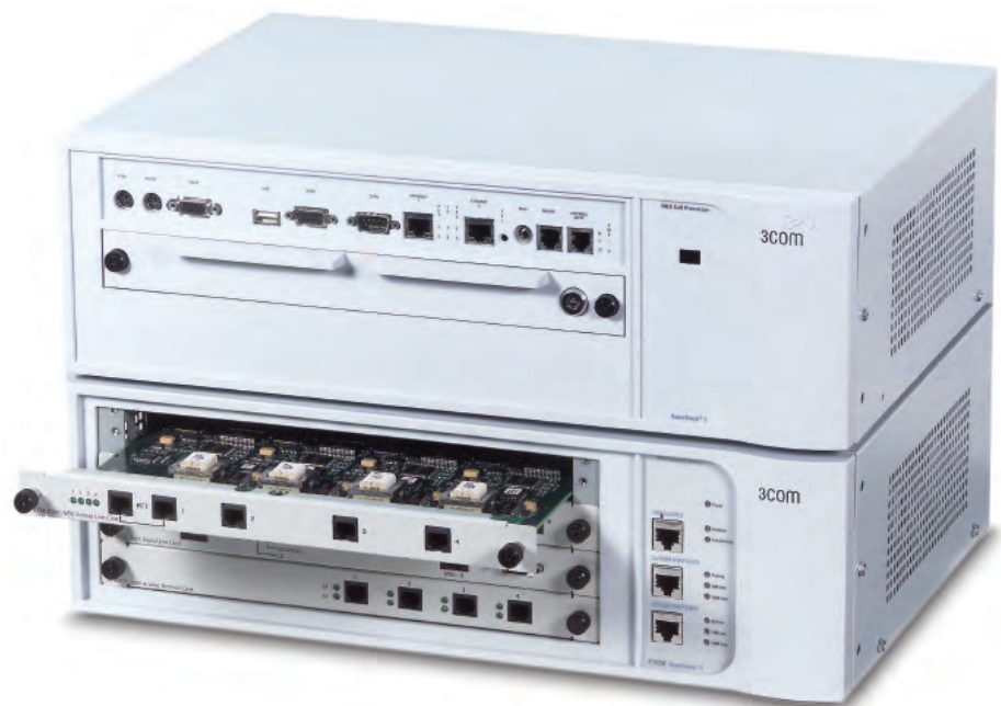
3Com SuperStack 3 NBX Networked Telephony Solution with the NBX V5000 chassis/call processor stack and an NBX Analog Line Card for convenient connection to the public switched telephone network. A number of interface cards are available for additional connectivity needs.
